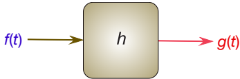
Figure 12.4 A schematic of an input signal f(t) passing through a filter h that outputs the function g(t) .
